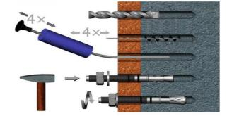
\*use the mechanical anchor M16x180 class 5.8
