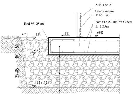
\*Foundation plate of thickeness 50 cm, concrete C20/25 W8. \*Layer of heat-weldable roofing membrane of thickeness at leasts 4 mm. \*Bedding concrete C12/15, thickeness of 10 cm. \*Crushed aggregate, fraction 0-32 mm, volume should be adjusted to the surface conditions. \*Subsoil
