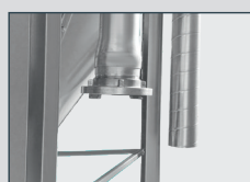
FEED TRUCK CONNECTION
